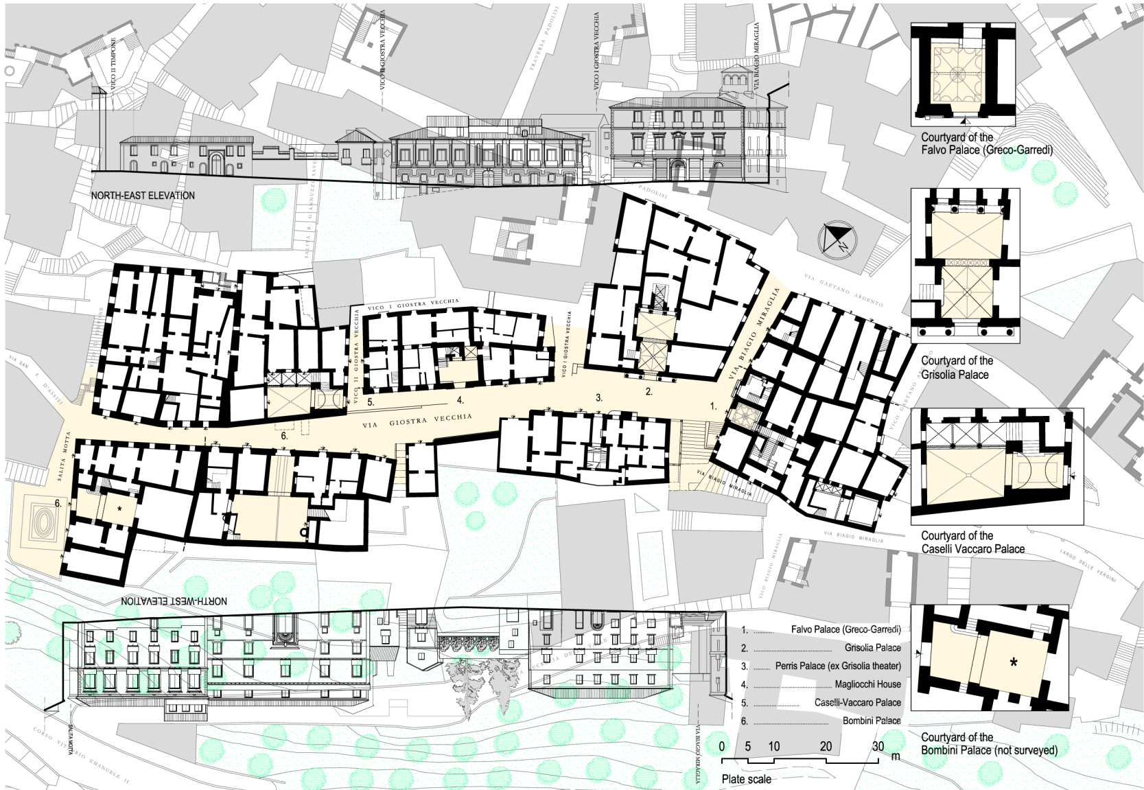
5. Plans and elevations of set of buildings in via Giostra Vecchia in Cosenza.
