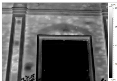
6. Thermographical investigation of Magliocchi House and Grisolia Theater; in the first façade, the investigation points out: masonry made of river pebbles with brickwork and stone blocks, on the ground floor and river pebbles with brickwork on the first floor; putlog holes set at regular intervals; brick relieving arches and wooden elements. The investigation of Grisolia Theater highlights: the reconfiguration of the façade (ground and first floor); river pebbles masonry and putlog holes; brick relieving arches and wooden architraves.
