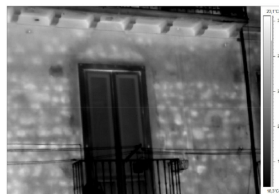
6. Thermographical investigation of Magliocchi House and Grisolia Theater; in the first façade, the investigation points out: masonry made of river pebbles with brickwork and stone blocks, on the ground floor and river pebbles with brickwork on the first floor; putlog holes set at regular intervals; brick relieving arches and wooden elements. The investigation of Grisolia Theater highlights: the reconfiguration of the façade (ground and first floor); river pebbles masonry and putlog holes; brick relieving arches and wooden architraves.
