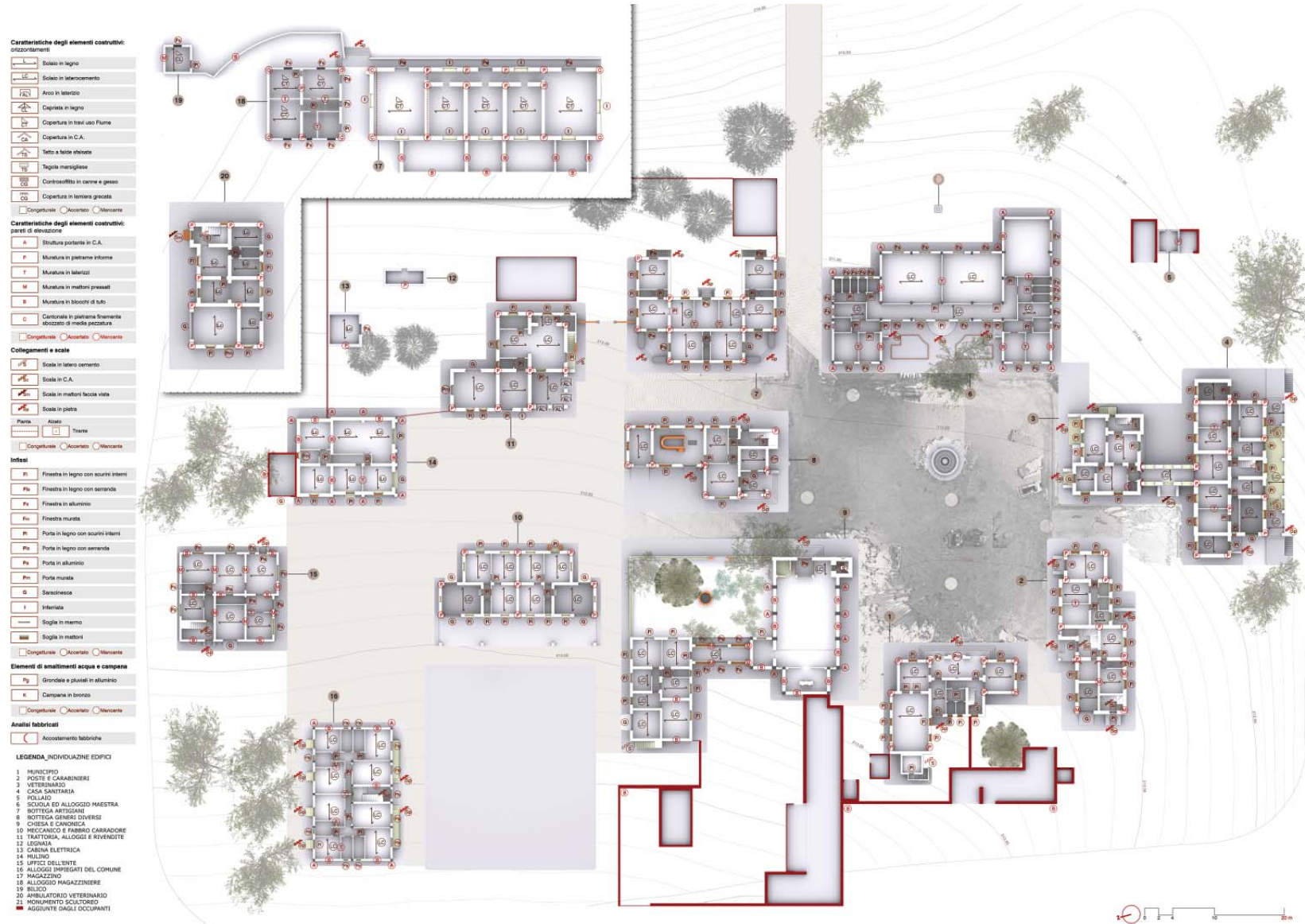
Fig. 12 - The graphic rendering of the ground floor plans with the indication of the functional distribution and the technical-constructive characteristics of the whole village.
