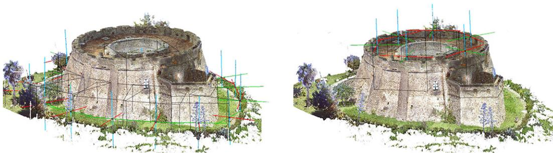
Fig. 4. 3D laser scanner survey. Images relative to the position of the scanner, respectively at the heights of 0.00m. and 11.20 m.
