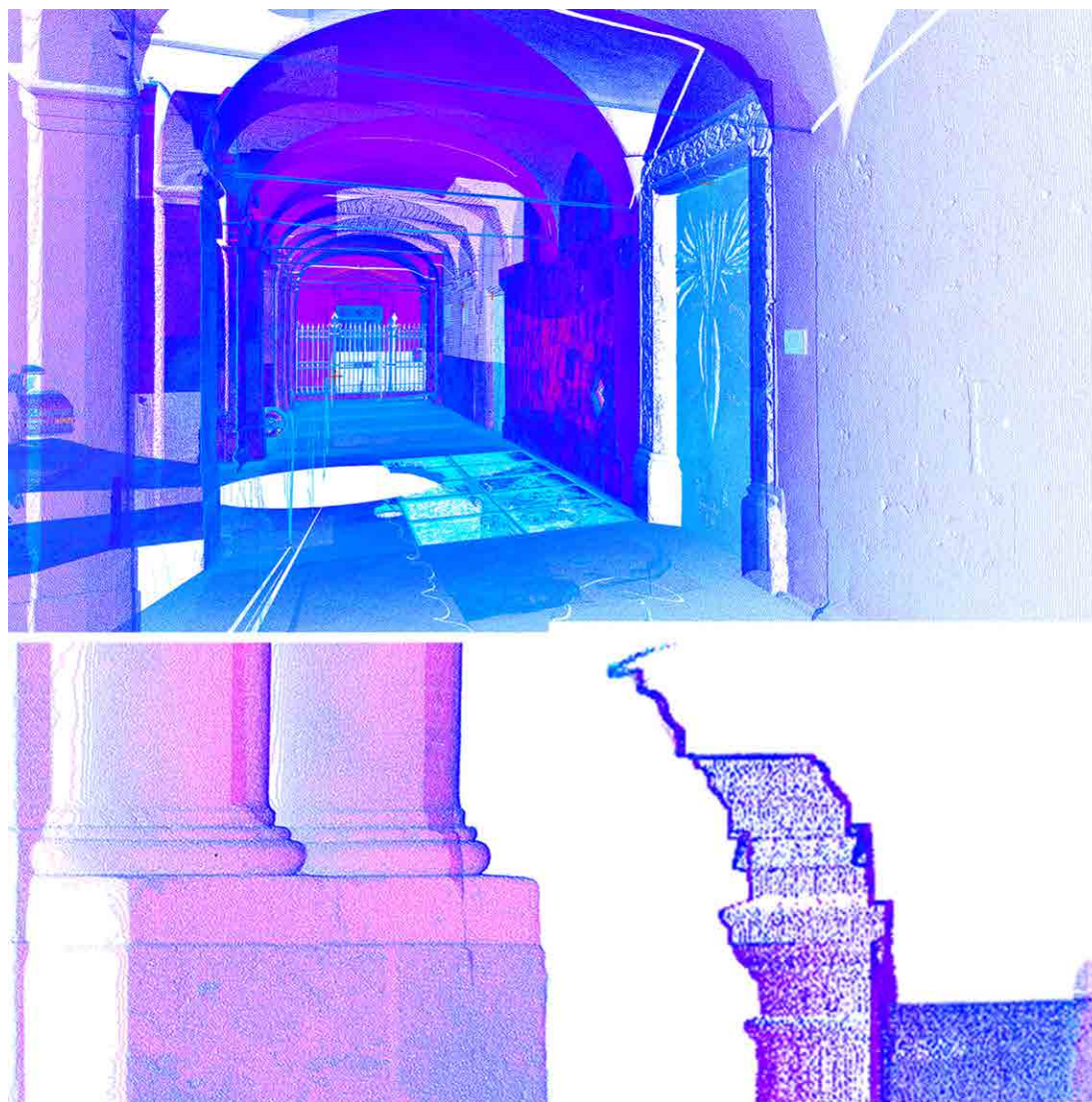
Fig. 10 - Numerical model of the whole cathedral and detail of the counterfaçade
