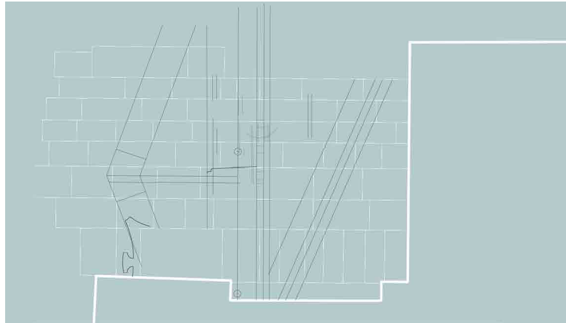
Fig. 4 - Graphic restitution of the layout with the location of tracing lines and travertine paving of the Mausoleum of Augusto.
