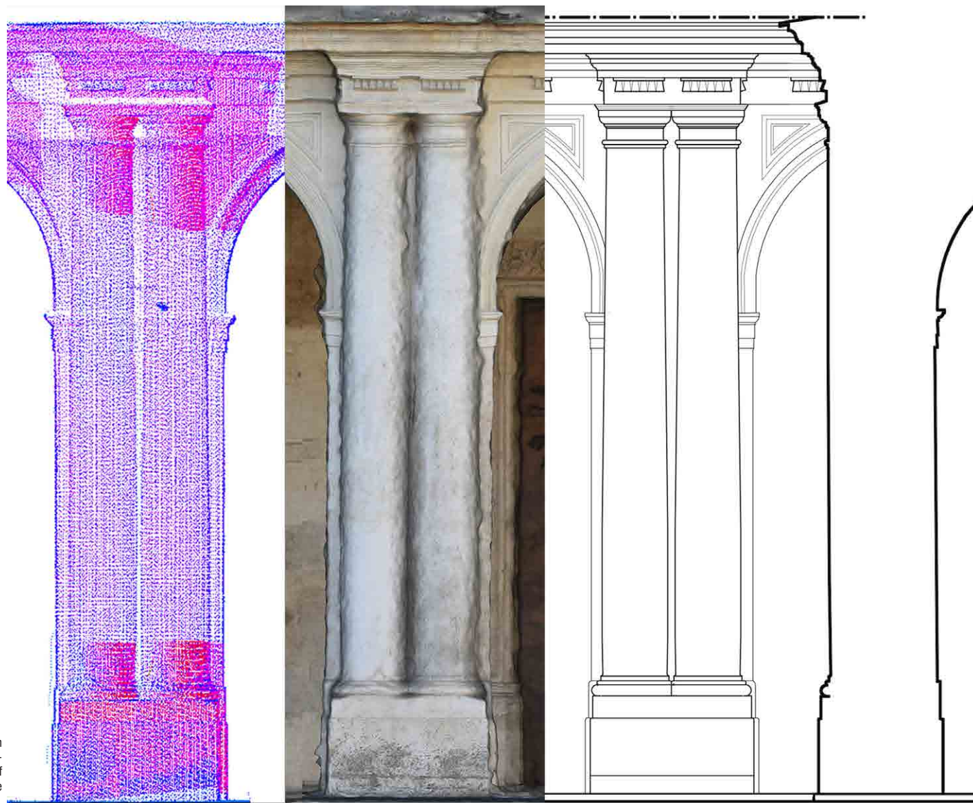
Fig. 12 - Data elaboration from 3D massive acquisition surveying for the construction of 3D/2D models of the binate column.
