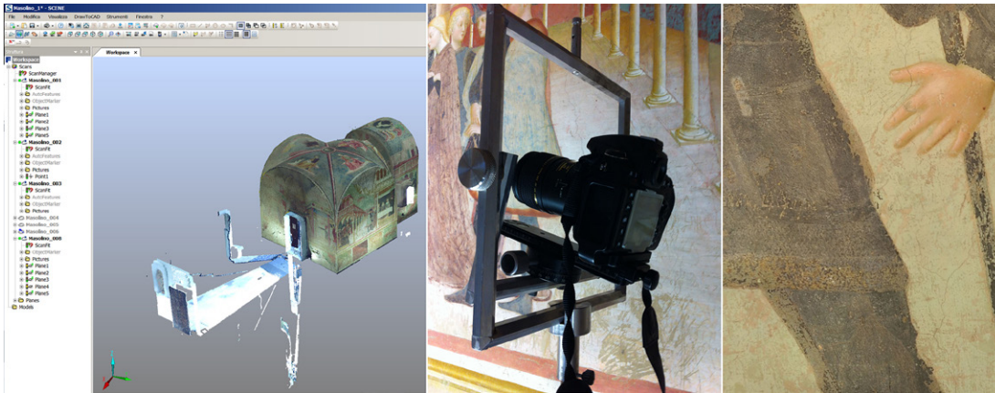
Fig. 3 On the left, the laser scanner points cloud of the Baptistery; in the center, the acquisition of the photos through a stand equipped with a calibrated rotating head that allows the camera to rotate around its perspective center; on the right, a detail of the orthophoto of the wall n. 9, made using grazing light.
