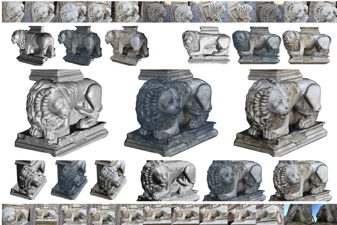
Fig. 18. Photomodelling for modelling the stilofori of Palazzo dei Priori in Perugia (Didactic composition by Francesco Andreoli, Matteo Scopetta _ University of Perugia _ Supervisors: Fabio Bianconi, Marco Filippucci).
