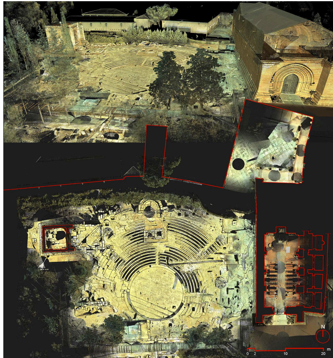
Fig. 2 - Readings of a stratified area. Planimetric and perspective views of a point cloud model of the Ekklesiasterion , of the Oratory of Phalaris and of the adjacent medieval and twentieth-century architectural structures of the upper Agorà of Agrigento (survey by M. Liuzzo, S. Giuliano, S. Savarino and E. Di Maggio).
