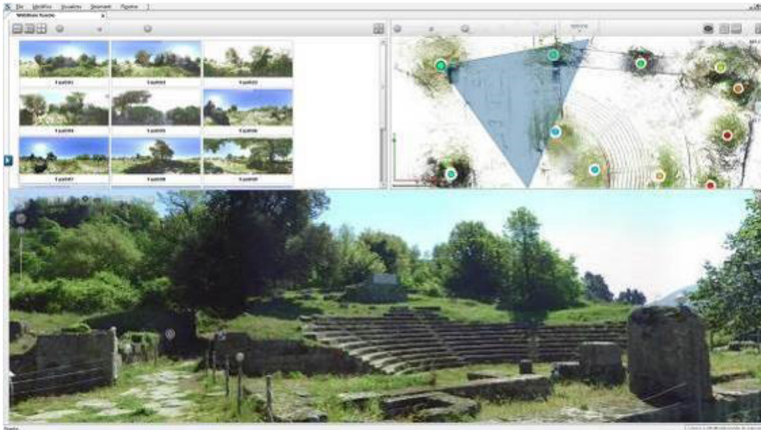
Fig. 6 - Navigation screen of the survey project with: scans preview, plano-altimetric stations layout and, in detail, panoramic image of the theatre and the via tecta ruins
