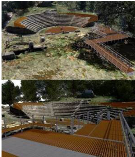
Fig. 11 - Some simulation render of the universal design of the archaeological park obtained by the integration between the area model (from survey) and the structures model (from design)
