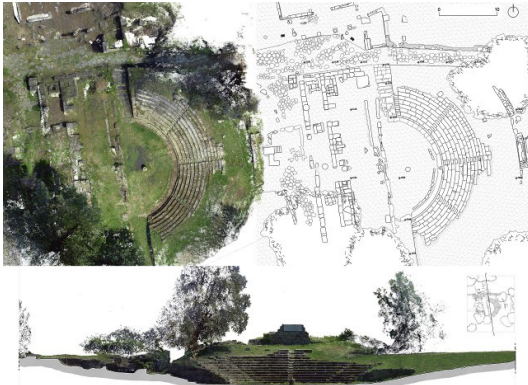
Fig. 9 - Top left and bottom, orthoimages from point clouds of the theatre (top and front views); top right, one of the graphic restitutions
