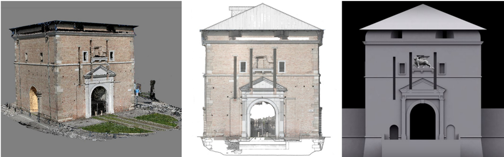
Fig. 3 - Photo Modelling of the external surfaces of Porta Pontecorvo, graphical restitution of the main prospectus (E. De Feo).
