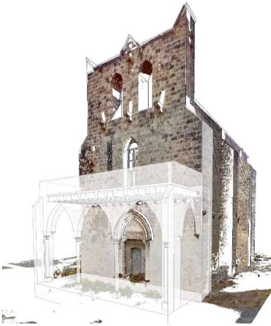
Fig. 9 - St. Anne, 3D model overlapping with the point cloud. Reconstruction of the west porch.
