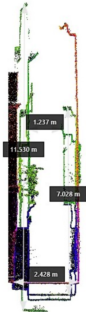
Fig. 6 - Point cloud overlapped cross sections showing extreme dimensions
