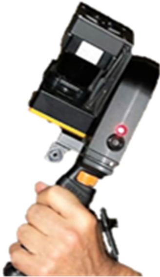
Fig. 4 - ZEB-REVO from GeoSLAM Scanner 3D provided by Geoavance S.L. Seville. Source authors
