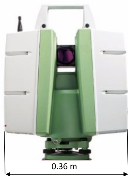
Fig. 8 - Leica C10 HDLS, provided by Graphic Engineering Department, University of Seville. Source: authors.
