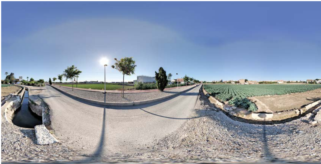
Fig. 7 - Equirectangular projection of a spherical panorama.
