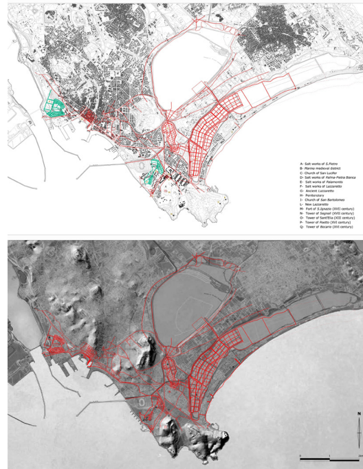
Fig. 15 - Graphic overlay between the "Plan des salines royales de Cagliari" and CTR-DTM (Regional technical Map and Digital Terrain Model) dated 1998 in scale 1:10.000. The compatibility between the documents allows the identification of historical buildings, the observation of coastline modification and to highlight the relationship between the salt works system and the morphology of the territory (graphic elaboration by Andrea Pirinu).
