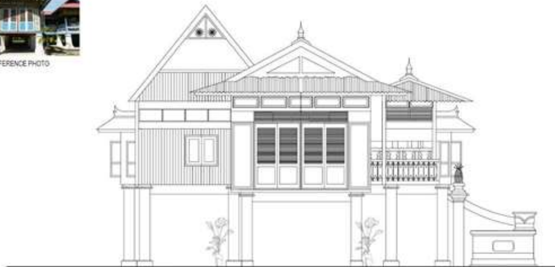
Figure 9a and 9b – Elevation drawings and views of Aristocratic Penghulu Ghani house, Merlimau Melaka, built in the 1800s yet regularly renovated until the early 1900s showing the essential Melaka style or syncretic Malay Chinese 'Peranakan' elements of Melaka (source: Applied Arts and Design students, IUM 2017)
