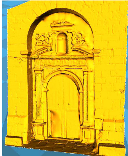
Fig. 10 - Image for direct 3D printing from the model obtained directly from the laser scanner mesh, without subsequent modelling.
