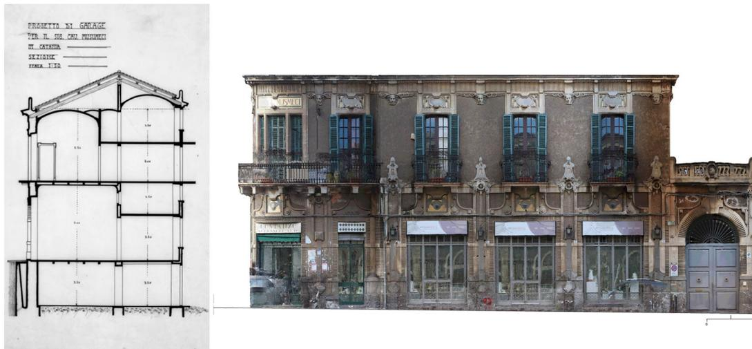
Fig. 7 - Garage Musmeci: project drawing of the cross section (on the left), orthophoto of main façade by polygonal model (on the right) (polygonal model by Ferrara E., Fichera A., Paladina G., Perrone V.)
