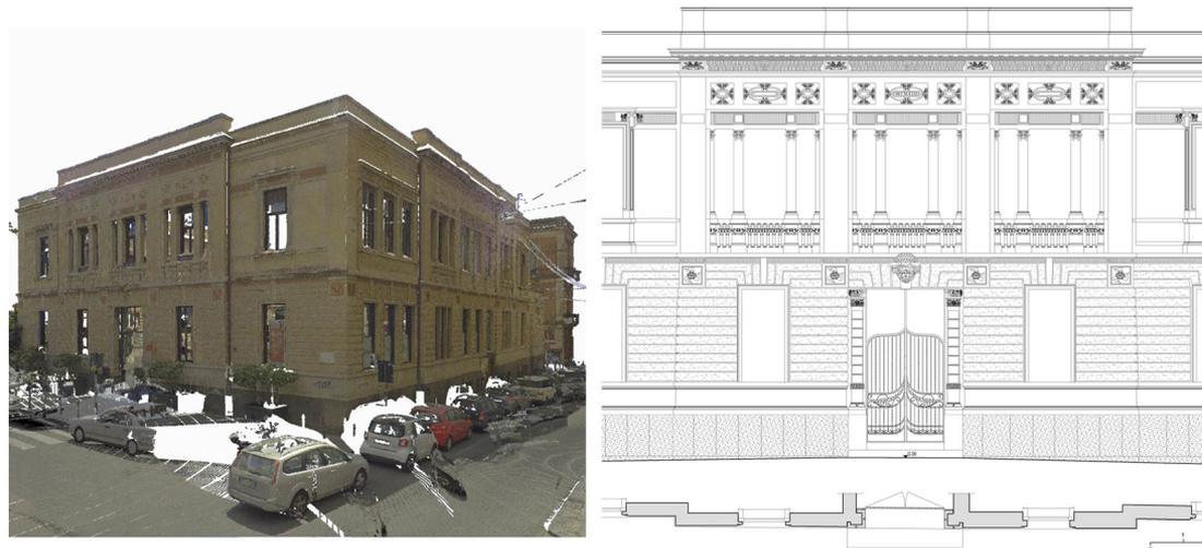
Fig. 3 - Palazzina Enel: view of the point cloud (on the left), main façade elevation (on the right) (2D restitution by Ardito G., Avanzato S., Balba A., Buscemi G., Cosentino S., Frazzetto L., Paganello F., Puccia D., Rapisarda D.)
