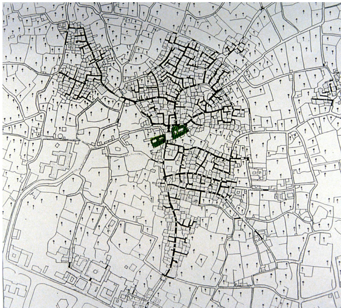
Fig. 11 - Ghadames, plan of the covered streets (in black). The small white squares are the light-wells that light special points of the streets, crossings, entrances of important houses, etc. (UNCHS - Habitat Survey Nov. 1987 U.M.)
