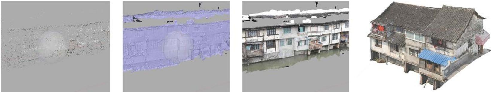
Fig. 5 - Development of 3D models of building units using SFM photogrammetry.
