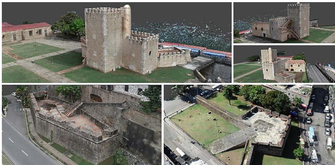
Fig. 7 - Point cloud obtained from the acquisition with UAV systems. Above the Fortaleza de Ozama , below: on the left the Bastion of the Invincible , on the right the Fuerte de la Concepcion .
