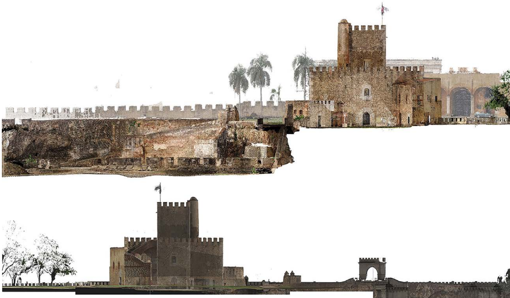
Fig. 6 - Point cloud obtained from the acquisition with TLS systems.
