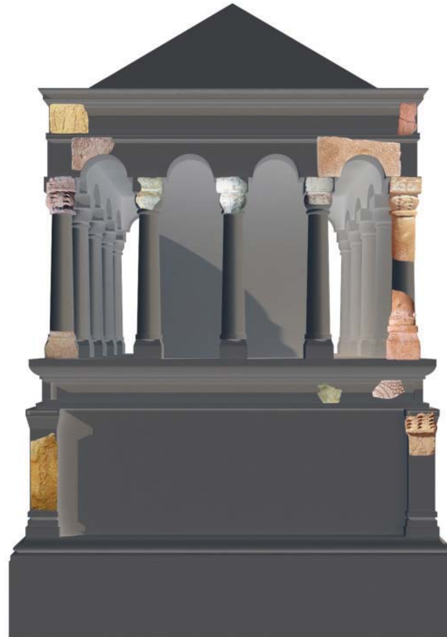
Fig. 52 - 3d model of a Ghadamsian tomb with the most significant stones conserved in Ghadames aimed at giving a plausible idea of the architectural apparatus of these aedicule Tombs (Elaboration arch. Christian Nardini).
