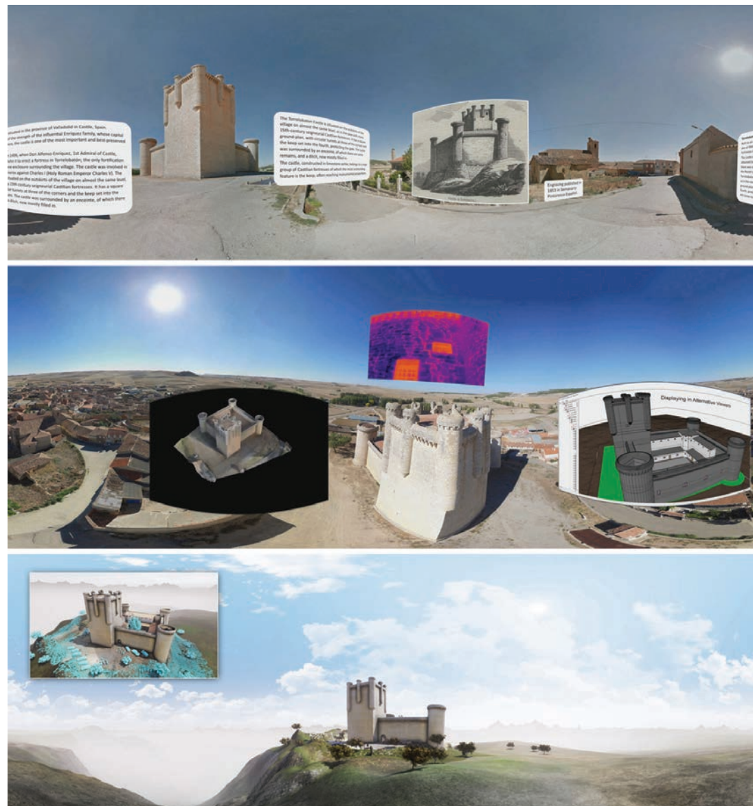
Fig. 9 - The 3D model of the Castle of Torrelobatón in Valladolid, Spain, was used to be linked to diagnostic tools, for documentation purposes and for creating an immersive environment, bridging the gap between XR environments for technicians and tourists.
