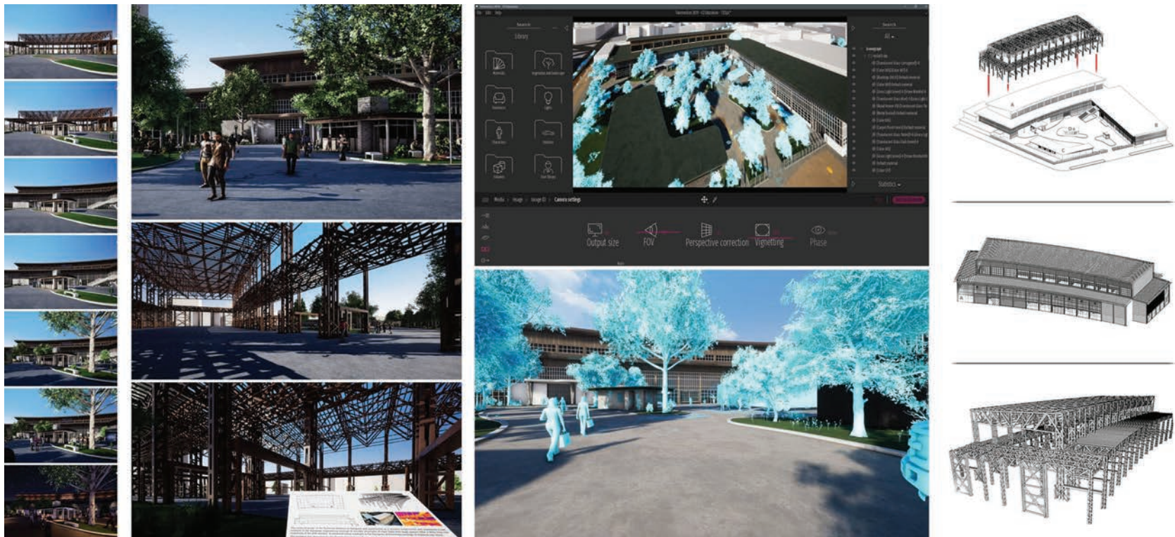
Fig. 7 - Through the use of the Twinmotion (Unreal Engine) platform, an off-site virtual reality navigation experience has been realized on the architectural complex of the museum in relation to its timber structure.
