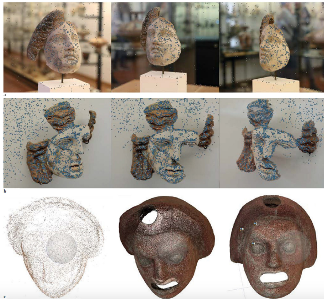
Fig. 7 - Automatic search for homologous points, (a) the Etairika teleion , and (c) the second Etairikòn teleion , (c) sparse point cloud, by A. Marraffa & F. Fatta, (2017).
