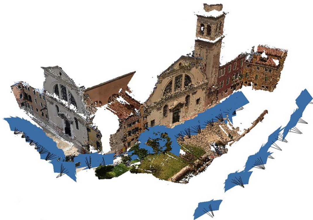
Fig. 3 - Exterior point cloud: camera positioning (Agisoft Metashape Professional software)
