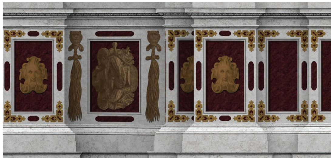
Fig. 7 - Detail of the 3D textured model of the proscenium with a reconstruction of repetitive geometric elements (pedestal).
