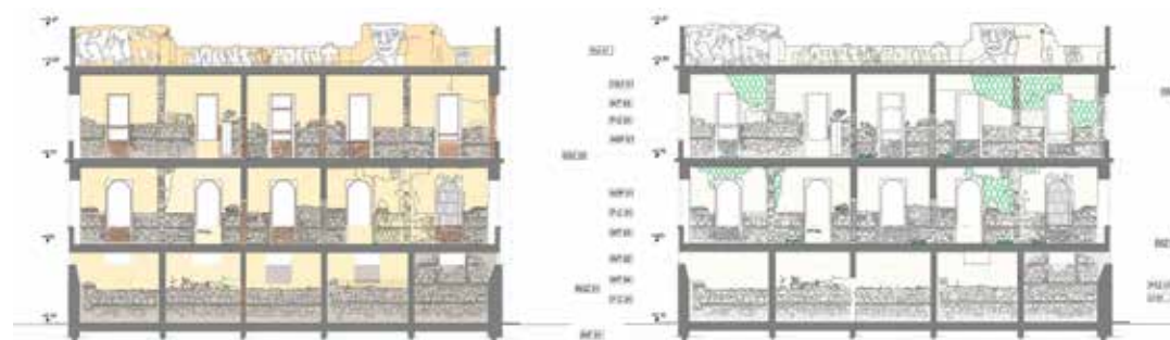
Fig. 17 - Material mapping on the left and mapping of the degrade on the right of the pavilion case study of the former general markets. The drawings were made by integrating the point cloud model, direct survey and orthophotoplanes.
