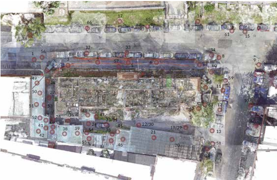
Fig. 10 - Position of the shooting points of the Laser Scanner campaign. Rework extracted from Autodesk Recap software.
