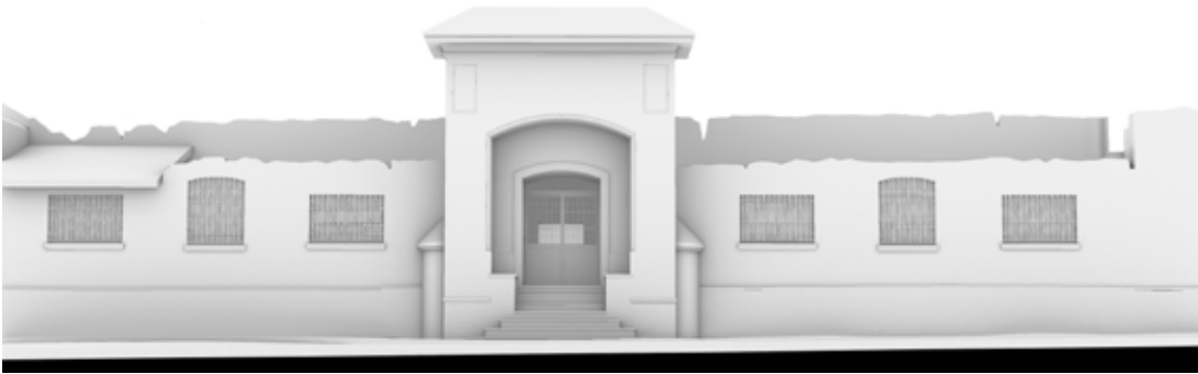
Fig. 9 - View of the three-dimensional model of the exfilanda pavilion. First NURBS model made from point cloud.
