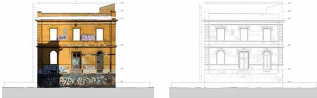
Fig. 16 - Orthophotoplan, and CAD drawing of one of the pavilions of the former Mercati Generali. The three-dimensional model of the point cloud was obtained through a photographic survey campaign and a photomodeling process.
