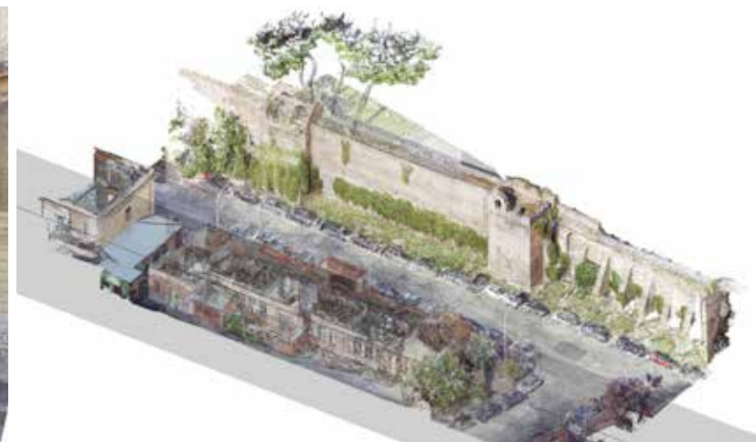
Fig. 12 - Isometric sectional view of the point cloud. The cloud is the result of the integration between the flight with the drone and the laser scanner survey campaign.
