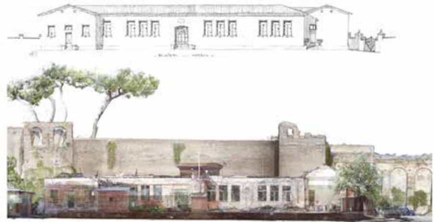
Fig. 14 - Comparison between the project design and the current situation obtained through an orthophoto of the internal courtyard. Note the addition of the accessory bodies dating back to 1965.
