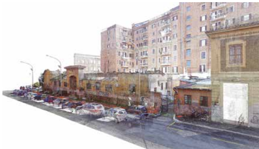
Fig. 11 - Perspective view of the point cloud. The cloud represented represents the first reworking, without considering the cleaning step of the disturbing elements.
