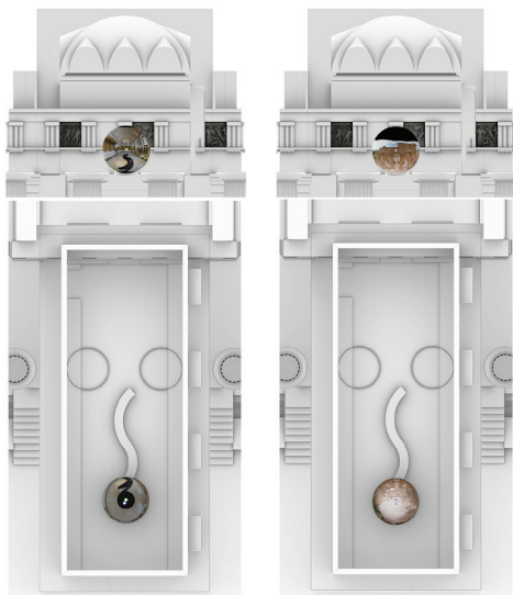
Fig. 13 - The spheres mapped with the equirectangular image of the Hall (left) and with the equirectangular image taken on site (right). The image shows that the deviation is absolutely acceptable for the purpose of the research.
