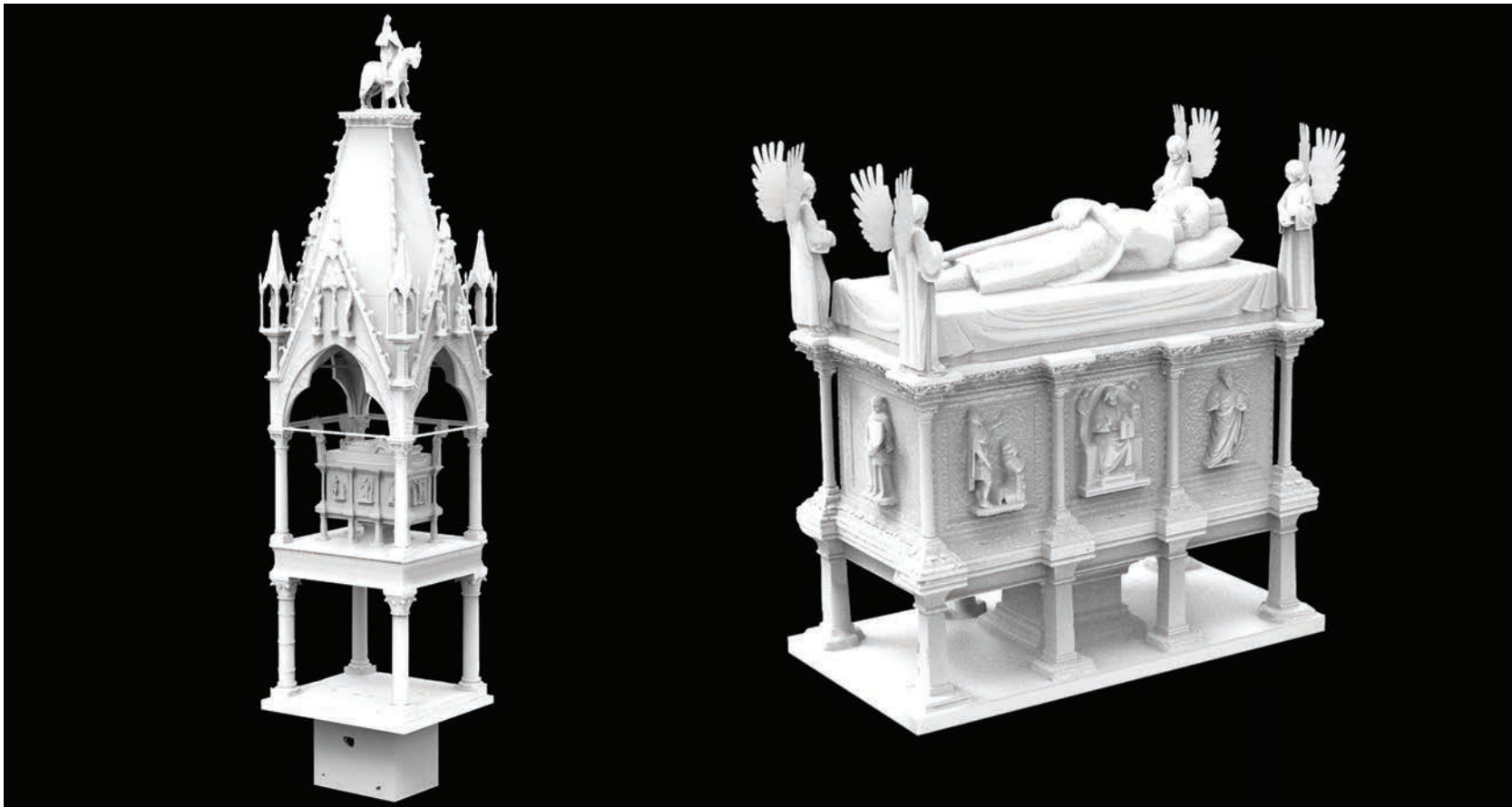
Fig. 17 - Three-dimensional print of the Ark of Mastino II in Verona in 1:25 scale. The starting mesh model, deriving from the integration of the laser data and the photogrammetric data from the drone, has been further discretized and lightened to allow for easy processing for printing. For the sarcophagus, given its high decorative characterization, it was decided not to simplify it completely, so that most of the decorations were visible.
