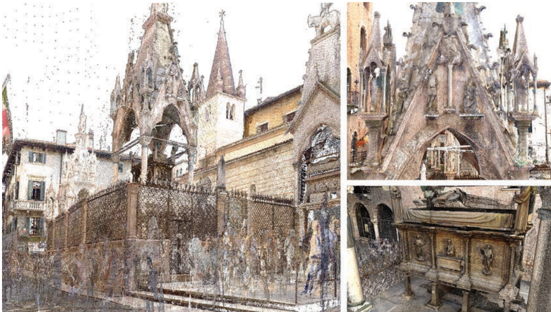
Fig. 5 - Views of the RGB colour point cloud obtained from the TLS survey.
