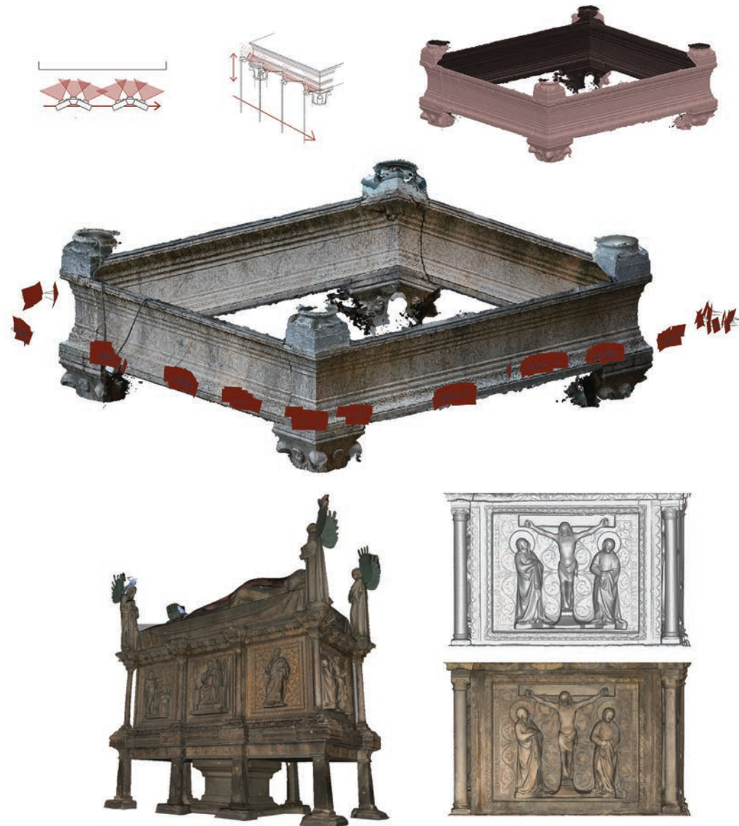
Fig. 8 - The 3D textured model of the sarcophagus obtained from the structured light scanner after the post-processing phase.
